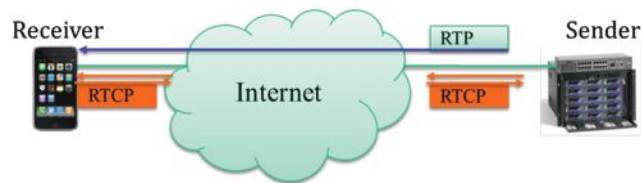
FIGURE 28.23 The bidirectional flow of RTCP packets.
