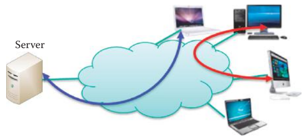
FIGURE 5.1 P2P versus Client/server networks: Blue line represents Client/server and red line P2P.
