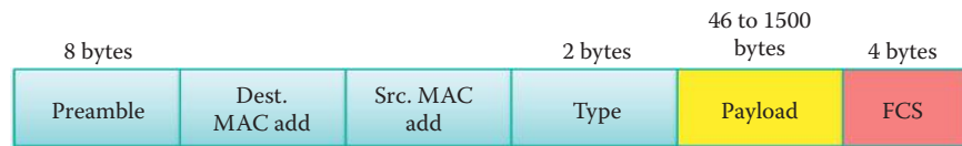
FIGURE 6.51 The DIXv2 Ethernet frame structure.
