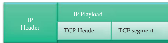
FIGURE 14.14 The TCP segment within the IP packet.
