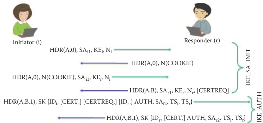
FIGURE 24.17 IKEv2 protocol with DDoS protection.
